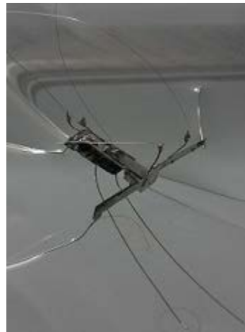
Fig 4.6.1 This robot has water-resistant legs to make sure it floats in water
